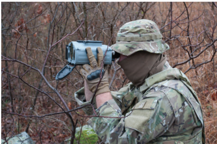
The Leonardo DRS Joint Effects Targeting System (JETS), shown above, is a next-generation hand-held precision laser targeting system. It has day and thermal night-vision sights, celestial compass sensors, an eye-safe laser range-finder, and a digital magnetic compass.
